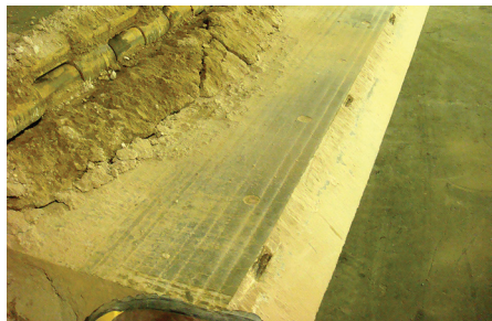
NanoSteel SHS 9700 overlay wear plate, 1/4" (6 mm) overlay on 1/4" (6 mm) substrate
