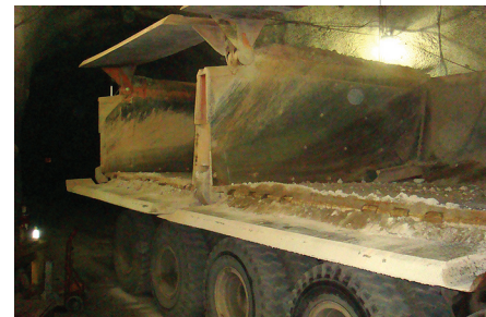
NanoSteel wear plates remain in service after hauling over 3 million tons in 28 months
