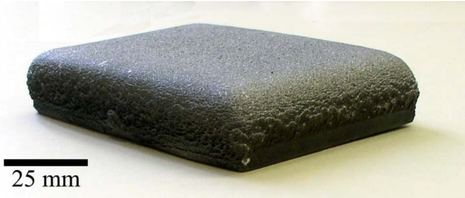
Figure 8 Optical micrograph of 800 mil thick SHS717 wire-arc coating deposited onto a ¼" thick 1018 plain carbon steel.
