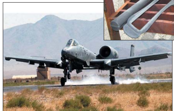
The A10 Warthog landing gear contains a piston made of the QuesTek Ferrium S53 alloy.
