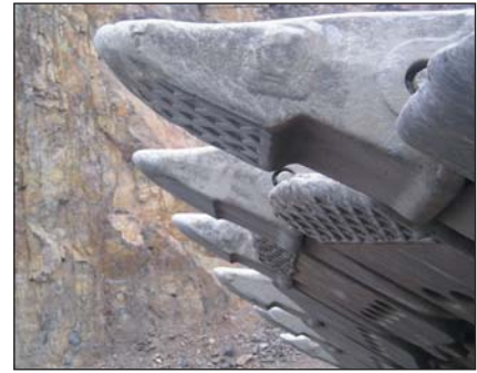
Left, a TEM micrograph shows the nanometer-size grain structure of one of NanoSteel's SHS alloys. Right, the SHS hardfacing applied to the excavator bucket tooth in the foreground provides a sharp contrast in wear protection when compared to bucket teeth in the background which have not been hardfaced.
