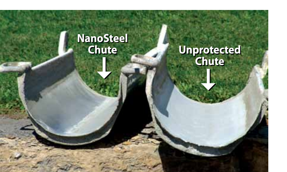
The unprotected chute shows severe wear from abrasion, leaks at the seams and must be removed from service.
