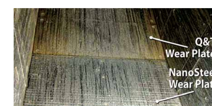
After deflecting 410,000 tons, NanoSteel overlay wear plate has exceeded Q&T plate life by 1.2x.
