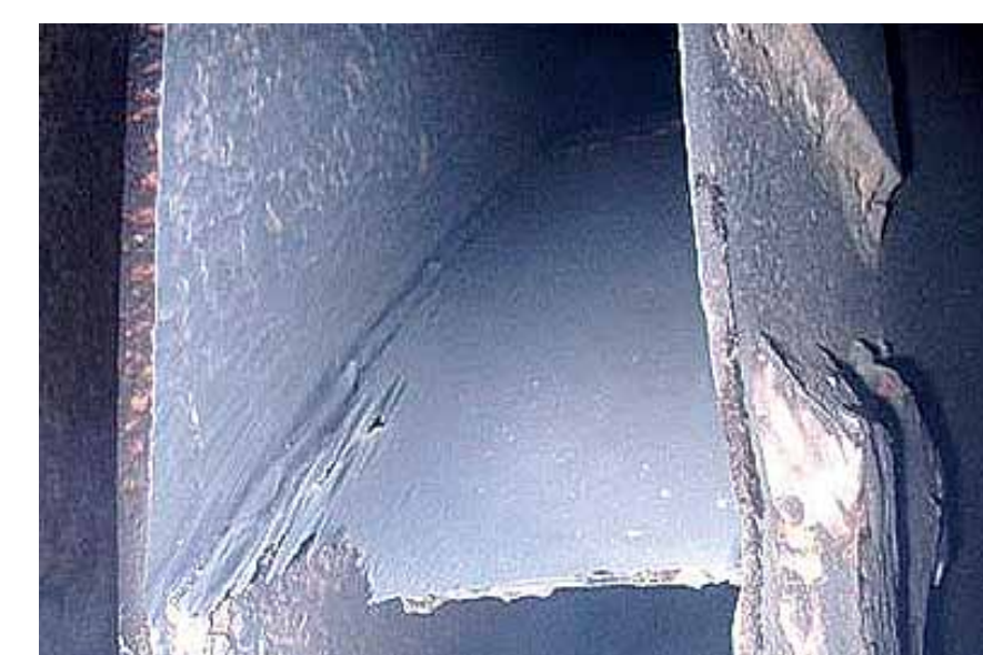
Unprotected steel fan blades are worn and must be replaced after 2-4 months of service.
