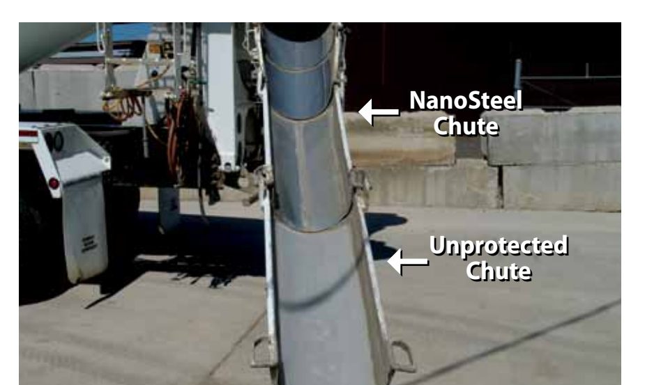
After 13 months in service, the NanoSteel chute has 75% of coating thickness present and the aluminum base is 100% intact.
