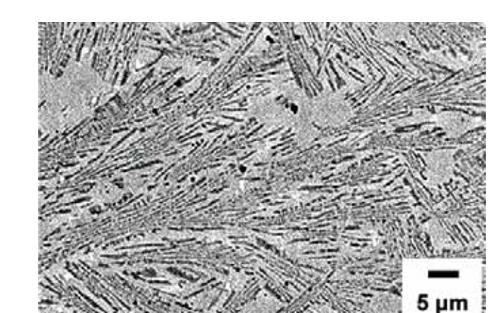
NanoSteel microstructure contains near-nanoscale (≤ 400 nm) grains.
