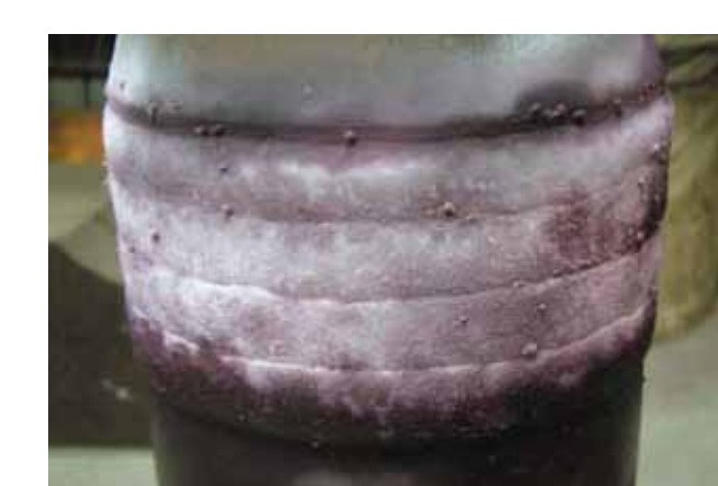
Dye penetrant testing proves the crack resistance of NanoSteel.
