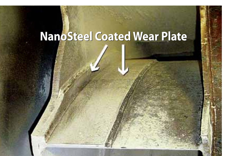
Fan blades with NanoSteel wear plate and thermal spray coating after 12 months of service.
