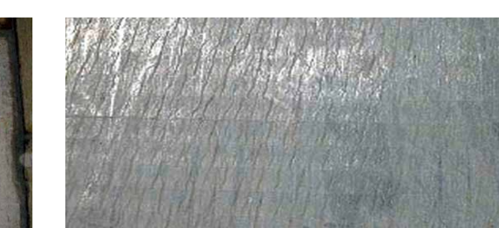
After deflecting 1,050,000 tons, NanoSteel overlay wear plate has exceeded Q&T plate life by 2.9x.
